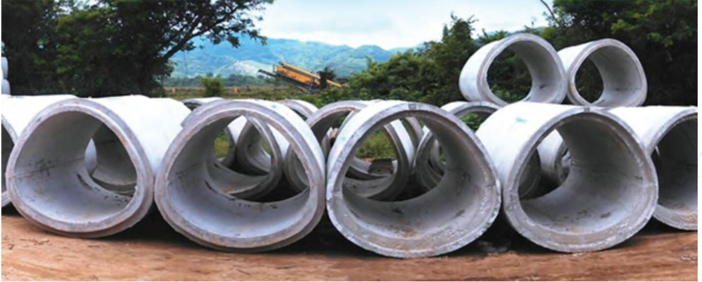
**Tubo TechSpan®** is a prefabricated reinforced concrete tube with vaulted sections that has particular designs for small cross structures like road sewers, culverts, any other utility pass, etc. To install the **Tubo TechSpan®**, a trench is excavated at the installation location as per the dimensions of the Tubo TechSpan®. Waterproof structures can be built using these segmental units.
