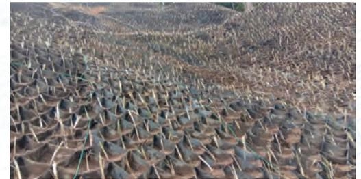
**ArmaWeb®** is a 3-dimensional soil stabilization and erosion protection system. It is made of High Density Polyethylene (HDPE) and welded at junctions to form cellular confinement systems. **ArmaWeb®** offers higher performance and faster installation for various applications.
