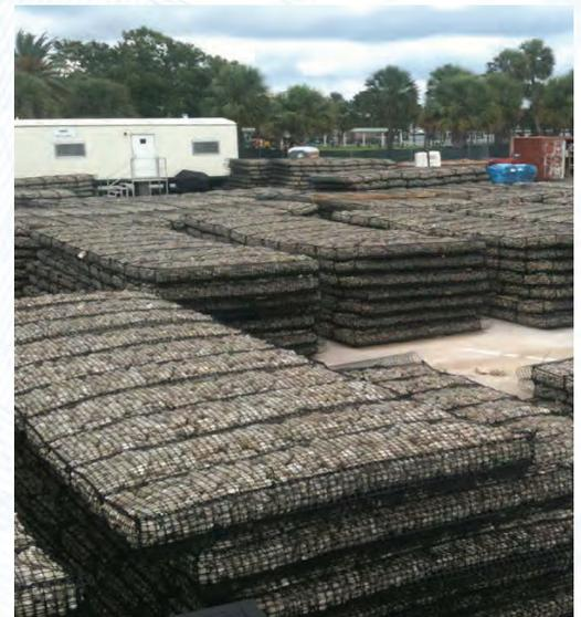
**TerraMattress®** is a corrosion free polymer based erosion control system designed to replace conventional rip-raps or wet stone pitching. This system is often used on slopes to construct boulder or soil in-filled semi-rigid crates and large bags to prevent water front induced erosion and provides protection against flash floods, moderate wave attacks and run-ups.
