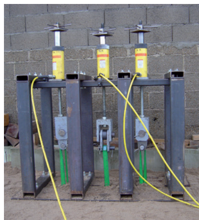
Strength testing the panels under the effect of the tensile load of reinforcements
